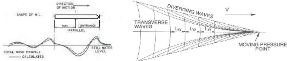
Figure 1. Left: Cross-sectional view of drawdown of water surface along vessel hull creating a long period wake. Right: Plan view of propagation pattern of diverging and transverse wakes (Herrington et al. 2009).
