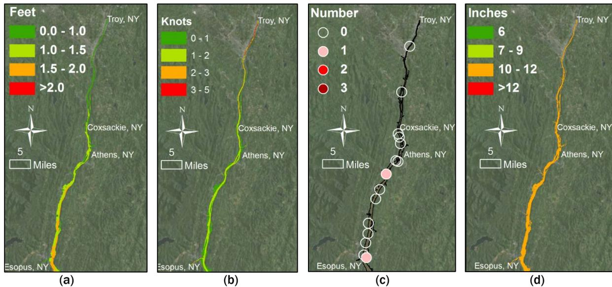
Figure 2: (a) Maximum wave heights in 2010; (b) Maximum current speed in 2010; (c) Observed number of wakes greater than 18.5 inches; (d) Daily ice thickness exceeded 5% of the time during the ice season, based on daily USCG observations over the 2005-2012 ice seasons (December-March) (Georgas et al. 2013).
