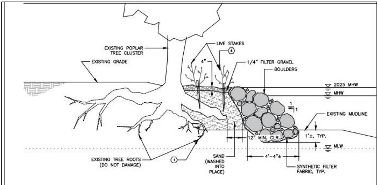
Figure 5. Design for stabilization of undermined poplar tree clusters at southwestern corner of site. The addition of fill and boulders up to the predicted 2025 MHW level will help mitigate erosion and protect existing poplars from further degradation for years to come. The planting of live stakes, using native species such as silky dogwood, red osier dogwood, and arrowwood viburnum, will help stabilize the soil and enhance the surrounding habitat. Credit: BlueShore Engineering.
