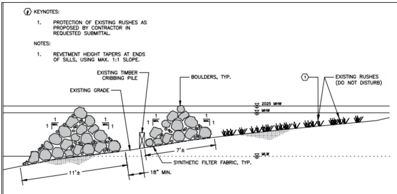
Figure 6. Design for the protection of existing rushes at the north of site. The addition of submerged stone sills up to the predicted 2025 MHW level will safeguard existing rushes from the full effects of wave action. Credit: BlueShore Engineering.
