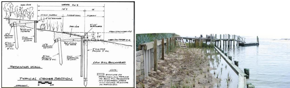
Figure 1. Typical New York low sill bulkhead and marsh project.
